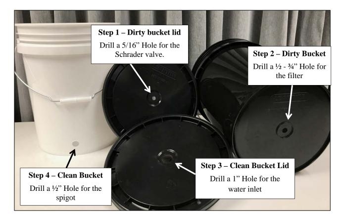
**Step 1**: Drill a 5/16" hole in the center of the dirty bucket lid to install the Schrader<sup>TM</sup> valve. Insert the valve into the dirty water bucket lid, making sure the rubber grommet passes through the hole and can be evenly compressed on both the inside and outside of the lid.
